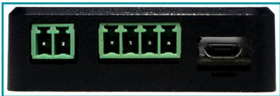
Caption: The side ports of the NIR 21IR are seen (connections for the Temperature Probe, the IR Extension, and the power supply).
