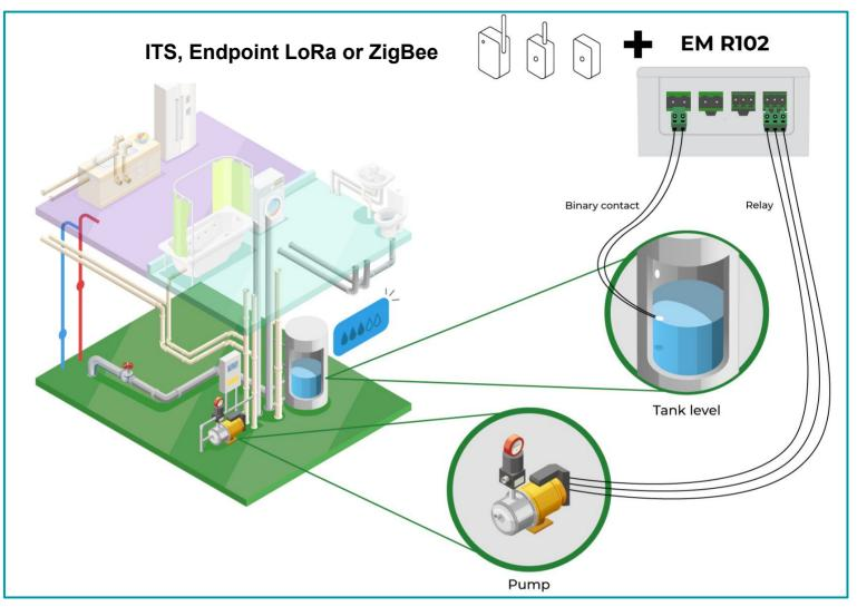
**Legend**: When it reaches a predetermined level of water in the tank, the extension triggers the pump.
