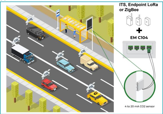
**Legend**: Attached to an urban structure, the sensor detects the amount of CO<sup>2</sup> present in the air and sends the data through the extension cable.
