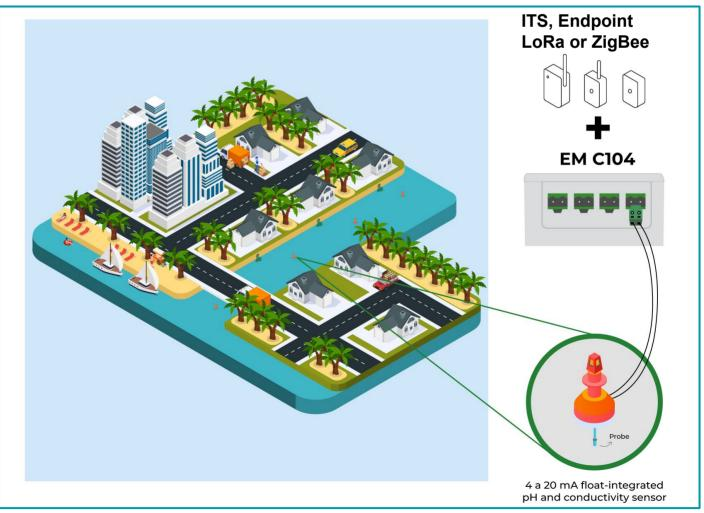
**Legend**: With the extender integrated into the sensor inside the float, it is possible to measure the pH of the water in that region.
