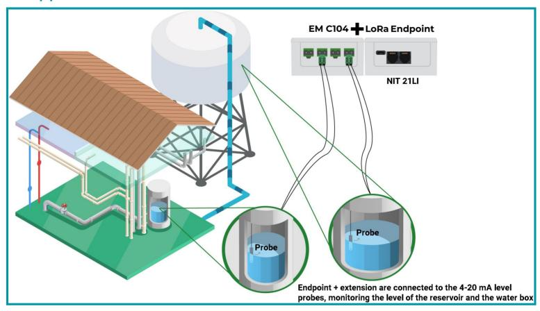
**Legend**: Association with level probes to check the volume of liquid in the reservoir and water tank.
