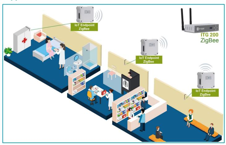
**Legend**: ZigBee endpoints in the hospital environment, monitoring three rooms and sending the collected data to the ITG 200 Indoor gateway.
