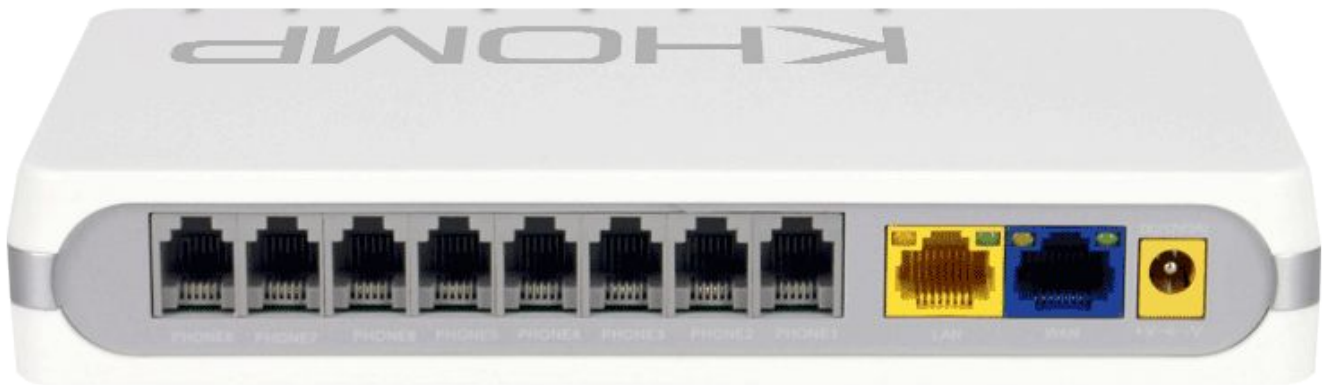
Rear view with FXS ports, LAN and WAN ports, and power supply input.
