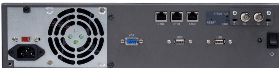
Visão traseira – Link E1/T1 com conector BNC coaxial
