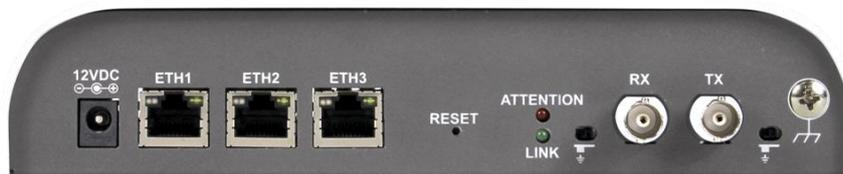
Visão traseira – Link E1 com conector BNC coaxial
