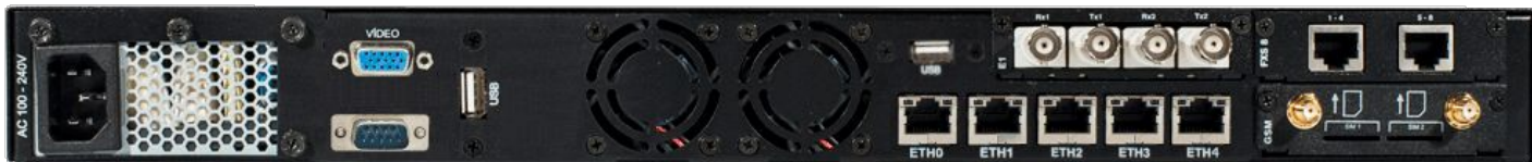
Subtitle: Rear view with 2 E1 Links (Slot1), 8 FXS (Slot 2) and 2 GSM (Slot 3).
