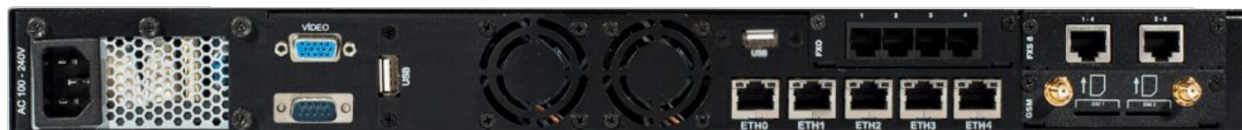
Subtitle: Rear view with 4 FXO (Slot1), 8 FXS (Slot 2) and 2 GSM (Slot 3).
