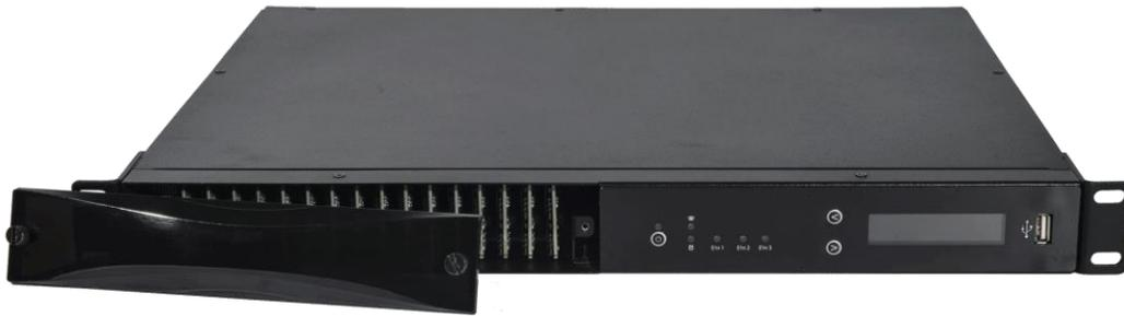
Front view with open cover for SIM card installation
