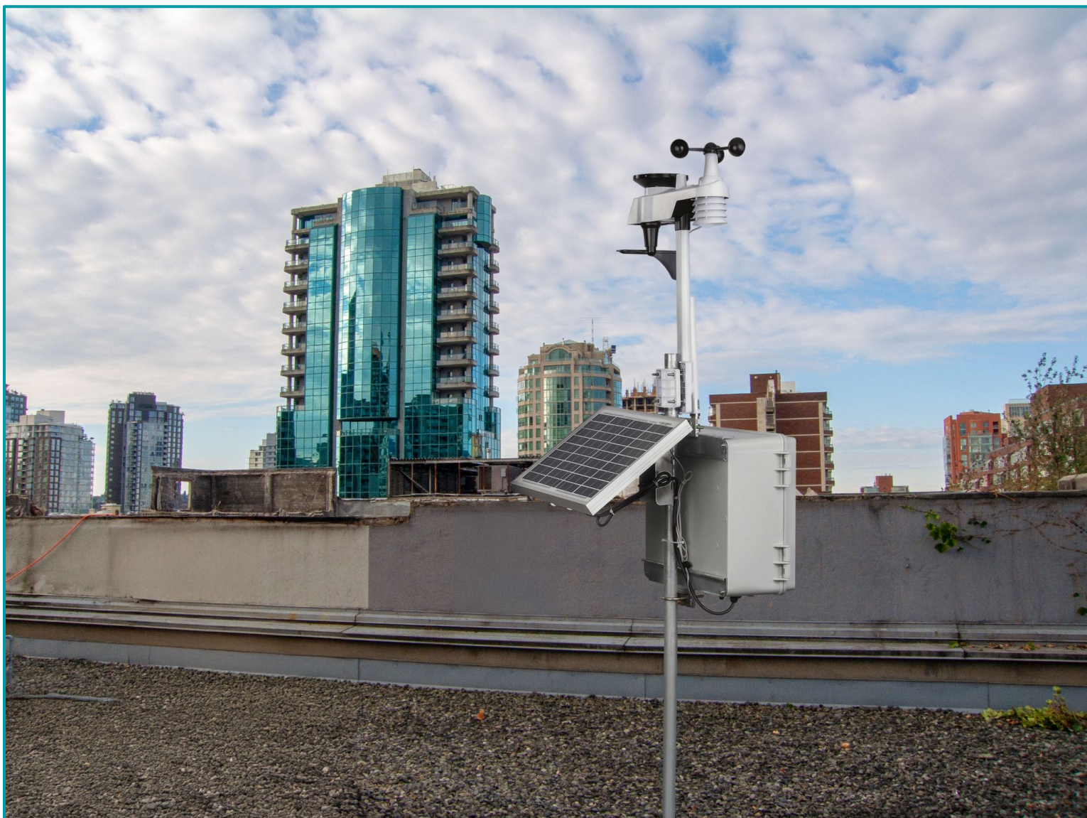
Legend: Weather Station sending city weather data for monitoring at the ITS .
