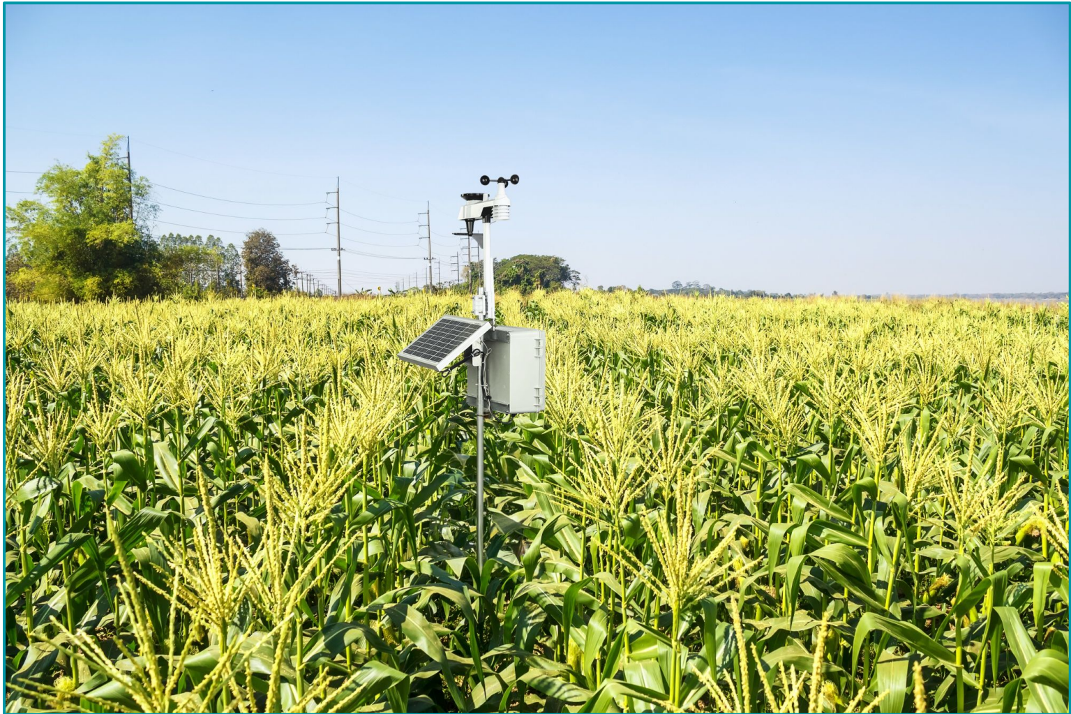
Legend: Weather Station sending farm weather data for monitoring at the ITS .
