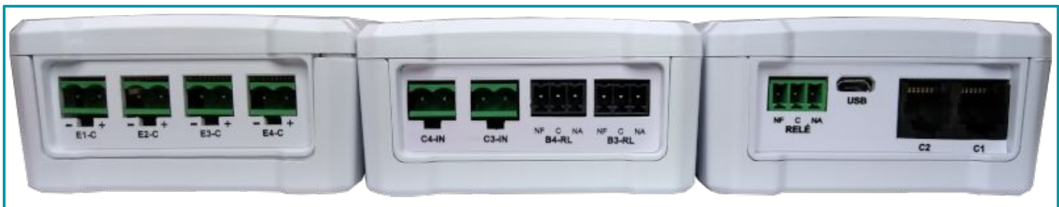
Caption: Ports view of the modular extensions EM C104 and EM R102, connected in ITS 402.
