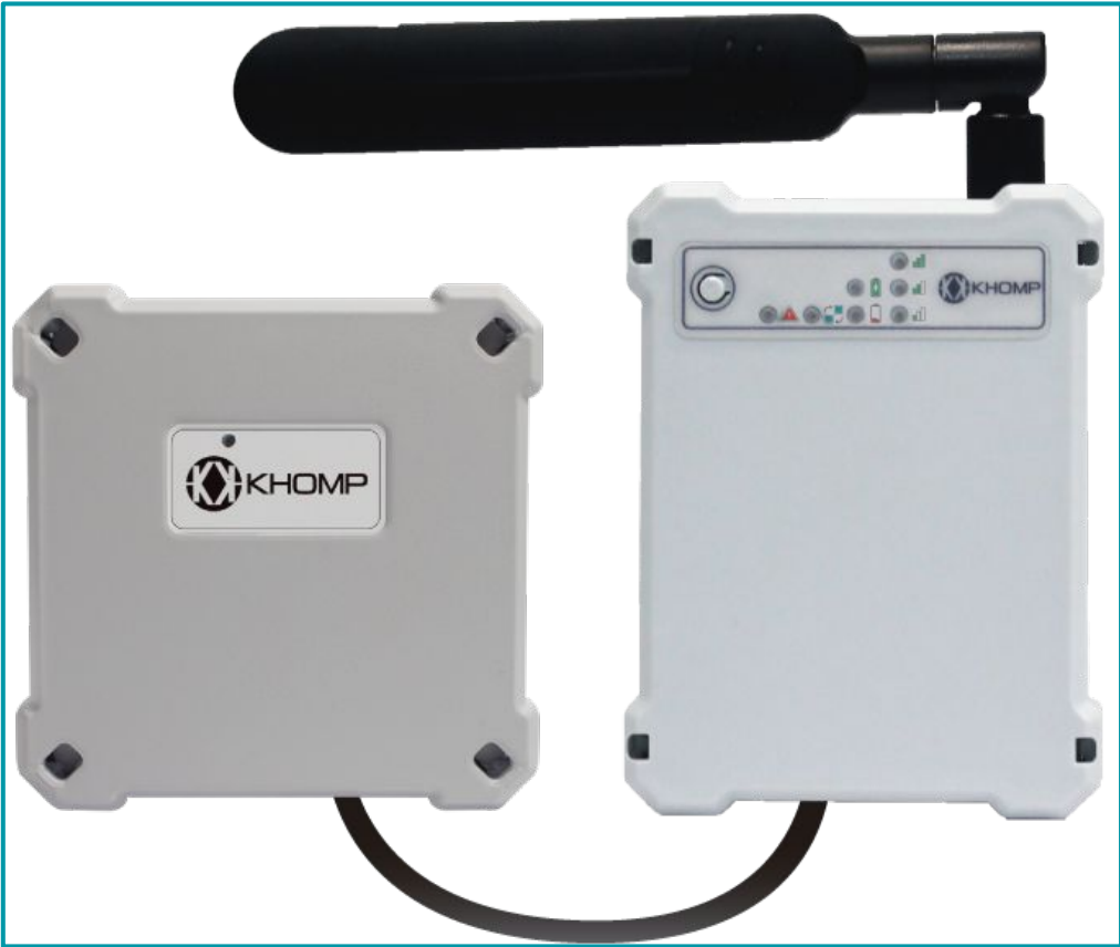
Caption: The modular extension connection is observed EM THW 200 on the side of the ITS to measure temperature, humidity, brightness and noise. The ITS 402 sends the data to the cloud/MQTT server via the indoor GSM antenna.
