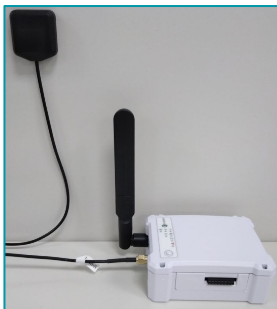
Caption: In the image, we observe the ITS associated with the External GPS Antenna , ideal for monitoring the delivery of goods by the carrier's truck.
