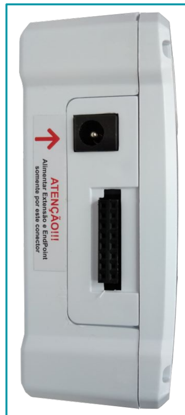
Caption: The image above shows the actual product set (ITS 402 is integrated into the R102 EM modular extension). The picture beside indicates the side of the modular extension EM R102, where there is the connector for system expansion and the place for connection of the power supply.
