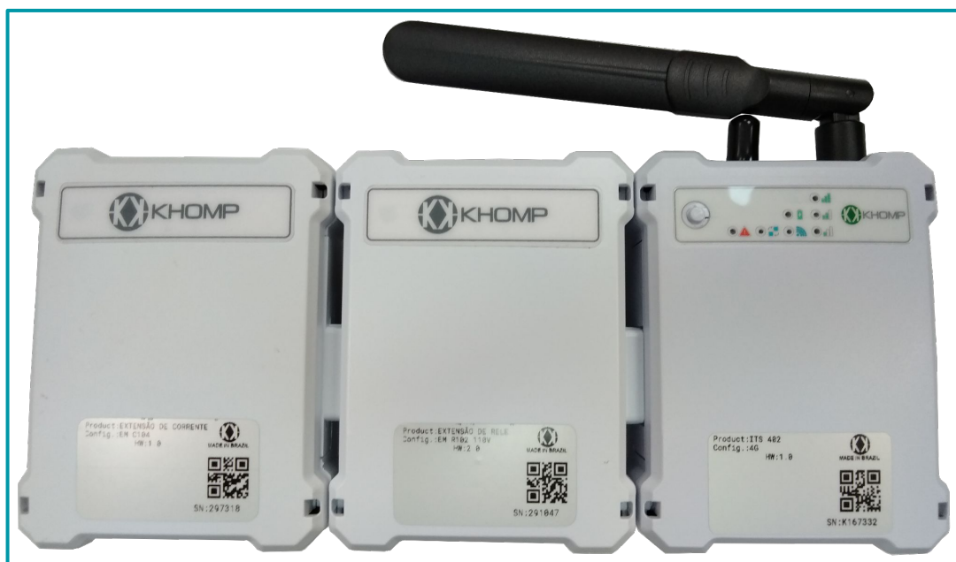
Caption: The image above shows the actual product set (ITS 402 is integrated into the R102 EM modular extension). The picture beside indicates the side of the modular extension EM R102, where there is the connector for system expansion and the place for connection of the power supply.
