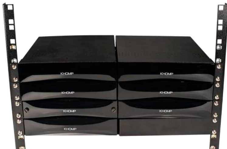
Example of 7 EBS modules arranged in a standard 19" rack
