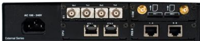
Example of assembly with 2 E1, 2 GSM and 4 FXO
