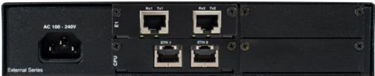
Rear view of model with 2 E1/T1 links (RJ45).
